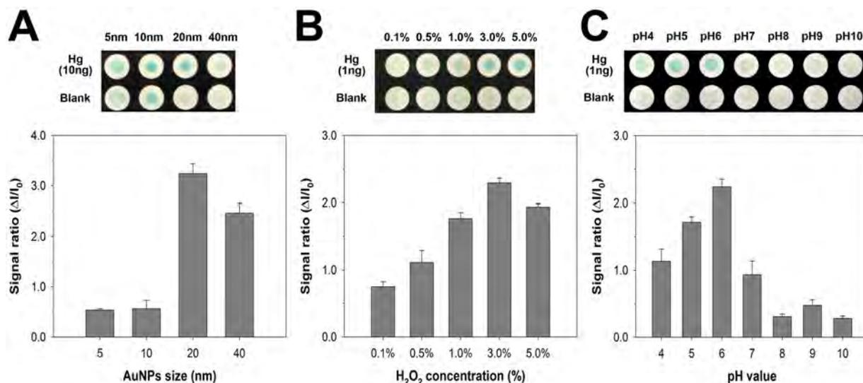
**Figure 2.** Effect of (A) the size of AuNPs, (B) the concentration of H<sub>2</sub>O<sub>2</sub>, and (C) the pH value on the colorimetric response in the absence and presence of Hg<sup>2+</sup> ions. Error bars indicate the standard deviation (SD) of three independent experiments.
