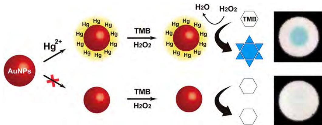
**Figure 1.** Schematic illustration of the AuNZ-PAD colorimetric sensing mechanism for  $\text{Hg}^{2+}$  ions based on the mercury-promoted nanozyme activity of AuNPs. When  $\text{Hg}^{2+}$  ions are introduced onto the AuNZ-PAD, the TMB- $\text{H}_2\text{O}_2$  catalytic reaction is highly enhanced by the formation of Au-Hg amalgam, resulting in blue staining of the paper chip.
