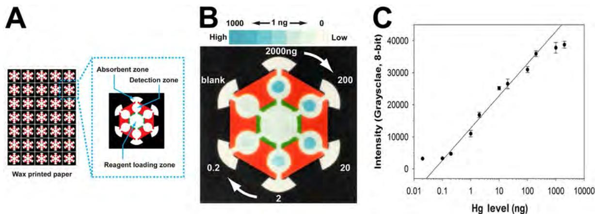
**Figure 3.** (A) Illustration of the AuNZ-PAD and its component parts. The white and colored (black, red, and green) regions represent the hydrophilic paper and hydrophobic wax, respectively. (B) Photographic image of an AuNZ-PAD used to simultaneous test samples with Hg levels ranging from 0.2 to 2000 ng. (C) Calibration plot of colorimetric responses for Hg levels in the range of 0.02–2000 ng. Error bars represent the SD of three independent experiments.
