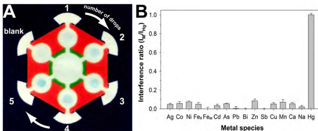
**Figure 4.** (A) Colorimetric signal amplification depending on the number of drops of test sample. A 2  $\mu$ L drop of test sample containing 0.4 ng Hg was repetitively applied on each test zone of the AuNZ-PAD with a time interval of 2 min. (B) Selectivity of the AuNZ-PAD against other metal/metalloid species. The added levels of Hg<sup>2+</sup> and other metal/metalloid species were 1 and 100 ng, respectively. Error bars represent the SD of three independent experiments.
